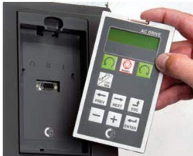
The removable control panel has a copy function that allows you to transfer settings to other Emotron FDU/VFX units.
