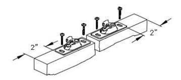
Also, for more even weight distribution of the Ball Bearing Rollers, have Two Wheels on one side, and Reverse the Wheels on the other Roller.
