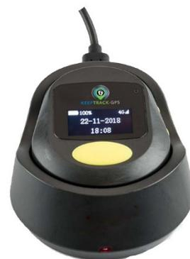
**1.4 The Screen:** Your screen shows the date, time in a 24-hour clock, battery level and signal. When you move the device around the screen will rotate with it, by pushing either the power or call button.
