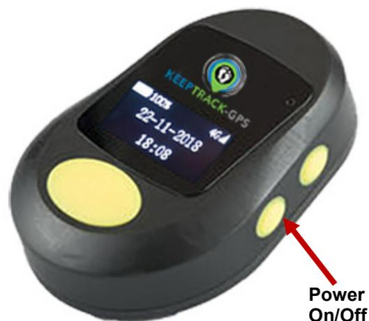
**1.1 Power on:** Press and hold the on/off button for 1-2 seconds, to power on the device, until you feel it vibrate release button and you hear it beep. The screen will show 'GSM Init' when it is powering up.
