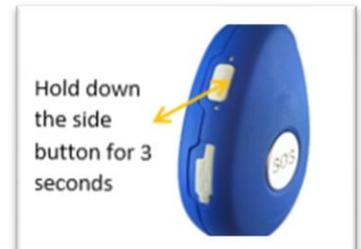
**1.3 Power off:** Press and hold down the side talk button and SOS button together for 3 second until all LED lights turn off
