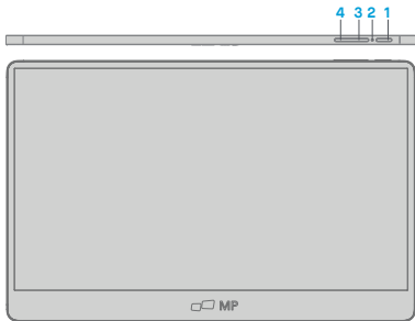
1 Up key 2 Down key 3 Power Button 4 LED Indicator
