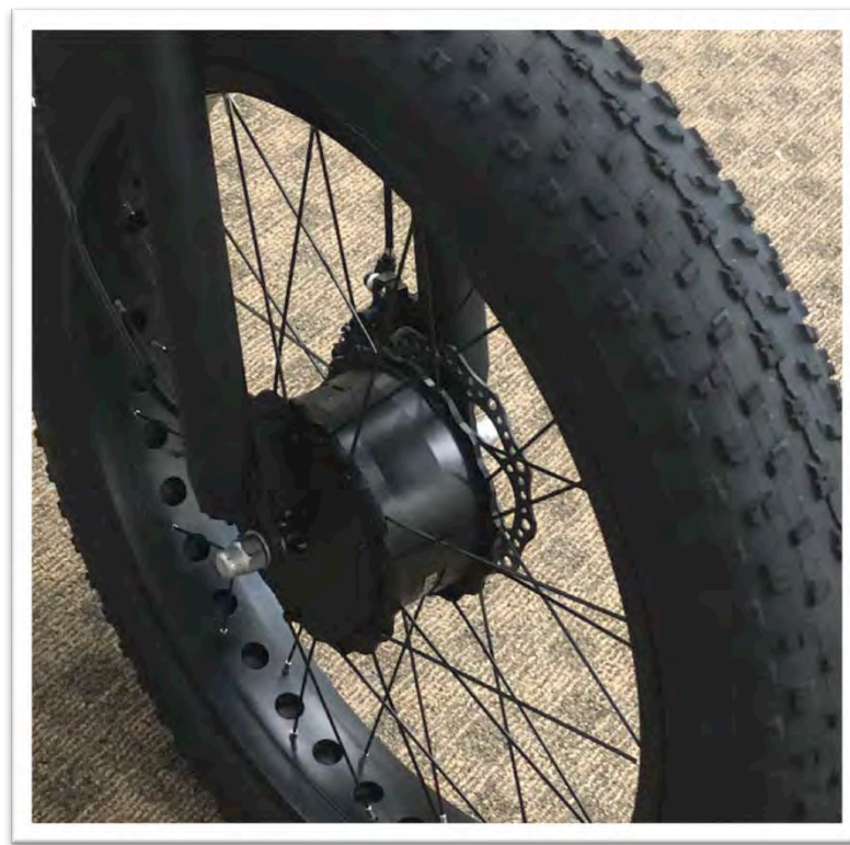
Front wheel already assembled into the fork.
