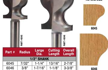
Use bearing (B16 for #6045, B18 for #6046) and Lock Collar (LC-1/2) on shank for template work.
