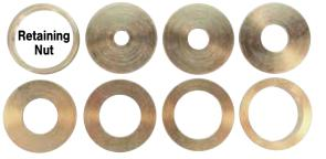
These solid brass inserts fit into your router base plate to reduce the gap around the router bit. Not only is this safer, but it also reduces tear-out and helps support smaller work pieces. Supplied in a set with openings of 1/4", 3/8", 1/2", 5/8", 3/4", 7/8", and 1", plus a retaining nut. Openings are slightly oversize for tool clearance. Fits any router with a standard 1-3/16" diameter recessed hole for template guides.
