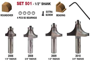
Roundovers are by far the most used edge forming bits in woodworking. This set offers the most common radii (R1/4", R3/8", R1/2") in 1/2" shanks, plus a hefty 3/4" radius workhorse. Extra bearings and wrench are included to convert each bit from Rounding over to Beading - i.e., Roundover with a decorative step.
