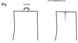
**#9.** Take the **pant front** pieces and form one pleat in each piece by folding the right notch at the top of the pant to meet the left notch. Sew this pleat down 1/4" away from the edge.
