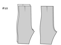
**#10.** Place one of the **pant front** pieces right side up in your work space. Lay the second pant front piece wrong side up on top. Match the curved crotch line, pin the two together at this line, and sew 1/2" away from the edge, trimming the seam allowance with your pinking scissors and pressing it open when finished.
