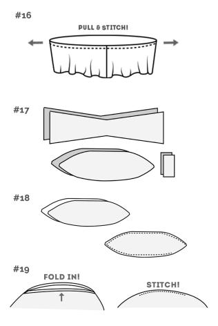
**#16.** Pulling the cuffs so that the elastic is taut, close the 2" gap you left open by straight stitching it closed. Make sure to hold your elastic and keep the cuff stretched out so the seam is straight! Clean finish the cuff seam allowance by trimming it with your pinking scissors.
