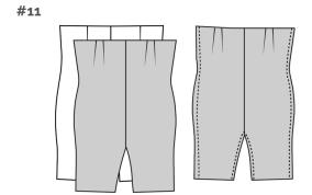
**#11.** Place the sewn pant front right side up in your work space. Lay the pant back wrong side up on top, matching the side seams. Pin the side seams together and sew both 1/2" away from the edge. Trim the seam excess with your pinking scissors and then press both open at the iron.
