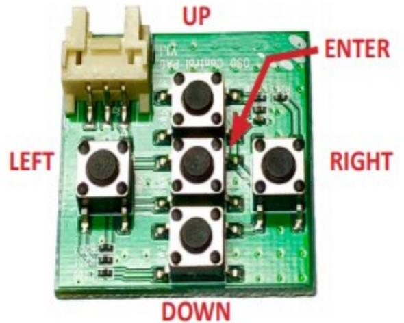
Use the OSD menu to make the necessary settings. Remember to Run **Save&Reboot** after the settings are made. Unplug the OSD Control Pad after setting the cameras and keep it in a secure location in case it is needed to change the settings.
