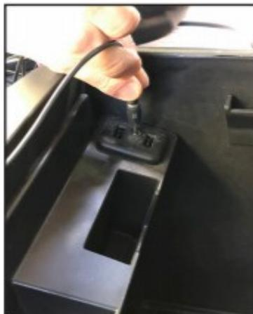
Plug in 3.5mm Aux Cable to factory Aux Input
