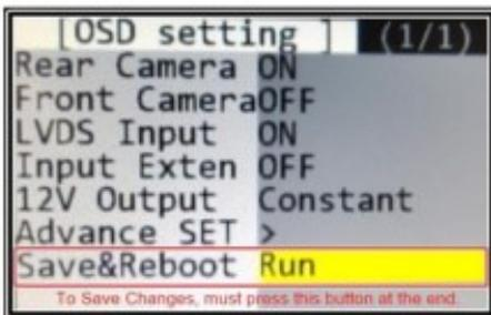
The front camera will automatically show on the screen when the gear is put to Drive from Reverse. Set the delay time on the OSD menu. Delay time can be set from 1 to 60 seconds after a putting the car to drive from reverse.
