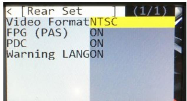
To turn ON the Dynamic Parking Guide Lines, go the Rear Input > Rear Set and turn ON Warning LANG. Go back to the root menu and Run Save&Reboot. Remember to unplug the OSD Control Pad otherwise the unit will not function properly. Set the parking brake on, start the car, put the gear in reverse, turn the steering wheel all the way to the left and all the way to right then put it in the center.
