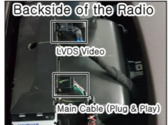
Plug and play connections behind the top side of the radio.
