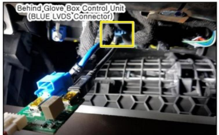
On RE models, the power harness is plugged in behind the headunit but the LVDS cable is plugged in at the HMI module (usually found behind the glove box).
