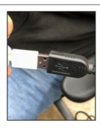
Plug in original smartphone cable to USB Ext. cable
