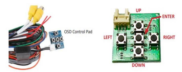
Use the OSD menu to make the necessary settings. Remember to Run **Save&Reboot** after the settings are made. Unplug the OSD Control Pad after setting the cameras and keep it in a secure location in case it is needed to change the settings.
