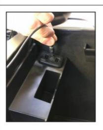
Plug in 3.5mm Aux Cable to factory Aux Input
