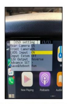
After plugging in the OSD controller, navigate down to *LVDS Input* and set to ON. Push RIGHT button to go to the next menu.
