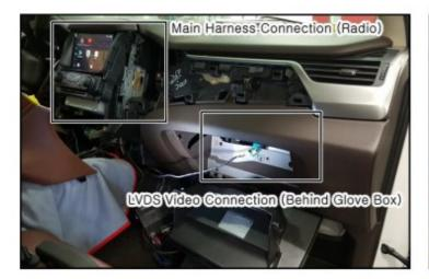
On RE models, the power harness is plugged in behind the headunit but the LVDS cable is plugged in at the HMI module (usually found behind the glove box).
