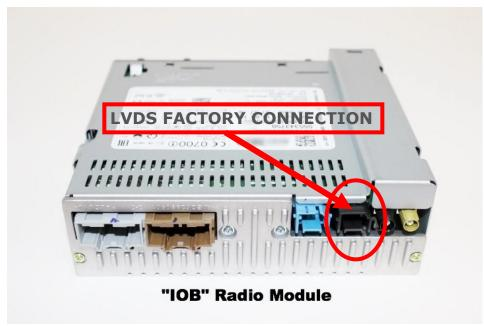
The IOB radio module is located behind the factory screen.
