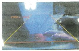
In TYPE, use  $\triangle$ ,  $\nabla$  on remote control, to select parking guide line Type for rear camera.
