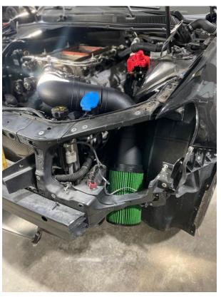
Put the coupler 4" x 5" coupler on the elbow that has the MAF housing and air straightener on it.
