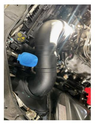
Install the filter. Now you can either remove the bumper to do this or you can work through the Fenderwell cover and install it all at one time.
