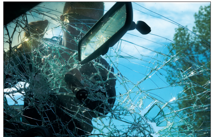
BreakAway attachments can break out windshields for emergency entry. Punch a large circular pattern with the BreakAway. The ceramic pins will penetrate the glass making it possible to break out the perforated area.
