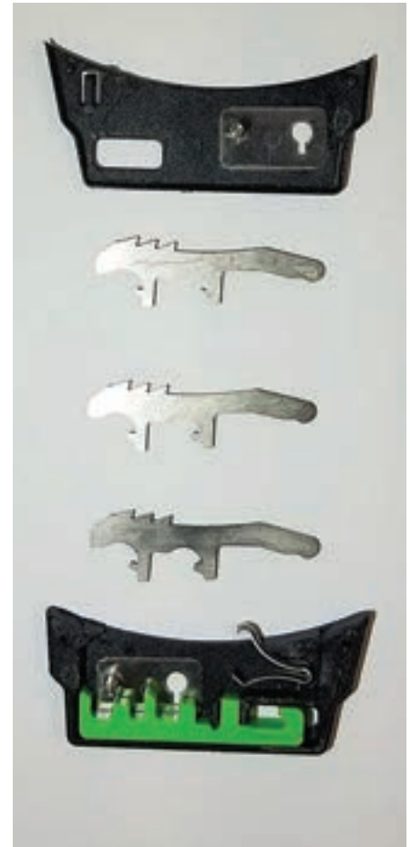
Figure 6. This is the triple pawl lockset.
