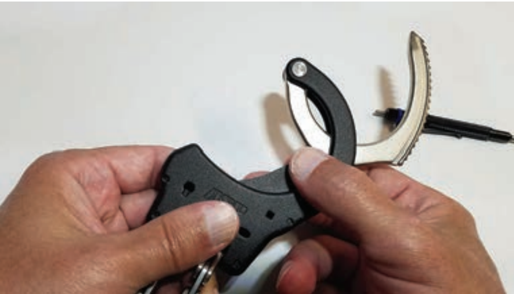
Figure 8. The lockset is levered up for removal.
