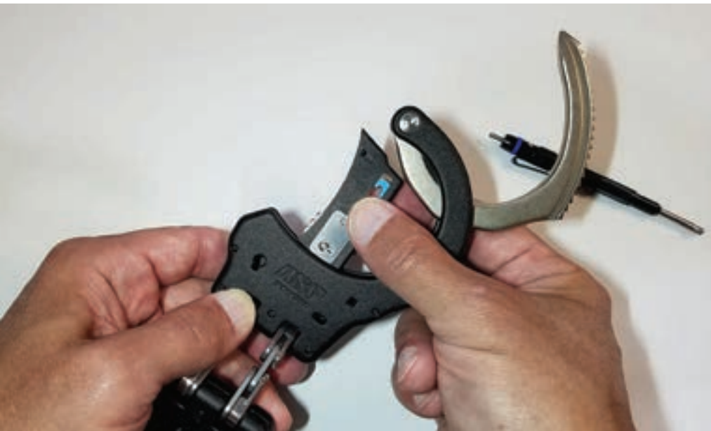
Figure 9. The lockset is removed and ready for replacement or service.
