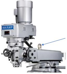
Step 1: The guard will install where the lifting eye bolt is on the top of the ram. If there is still an eye bolt in there, remove it.
