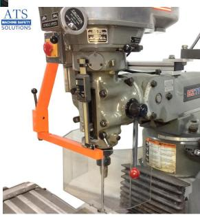
Step 7: With the guard closed, rotate the entire ram mount assembly until the orange front shield arm is square to the table of the machine.
