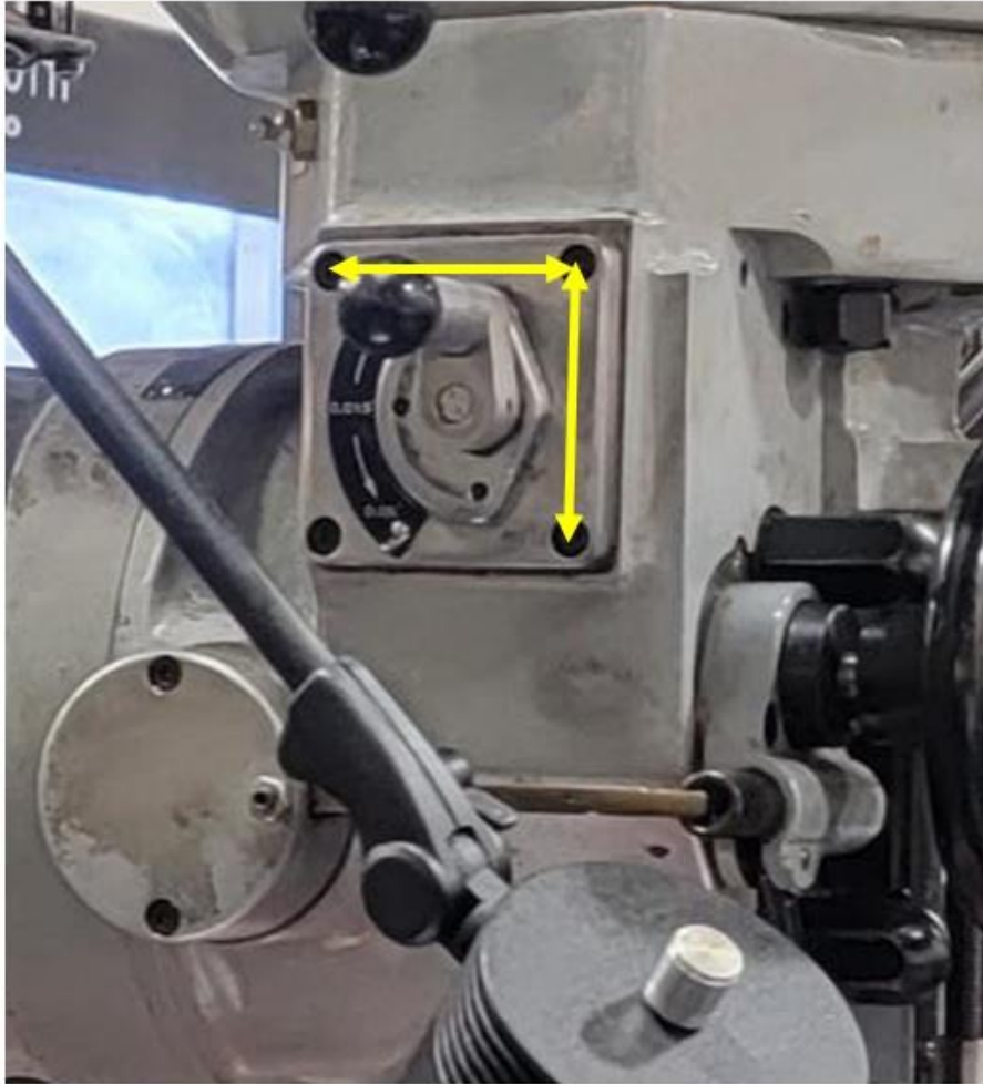
Part # MG-2 2.5" square bolt pattern Note: our mounting plates are slotted and will accommodate up to 2.75" square (70mm) bolt pattern Fits 95% of milling machines
