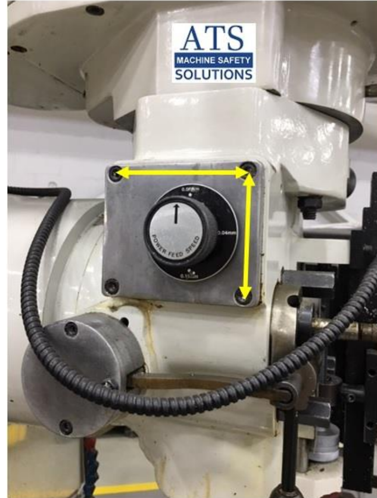
Part # MG-2T 3.0 x 3.5" bolt pattern This bolt pattern is used on some TRAK DPM machines, Milltronics MB-series and Clausing Bed Mills.
