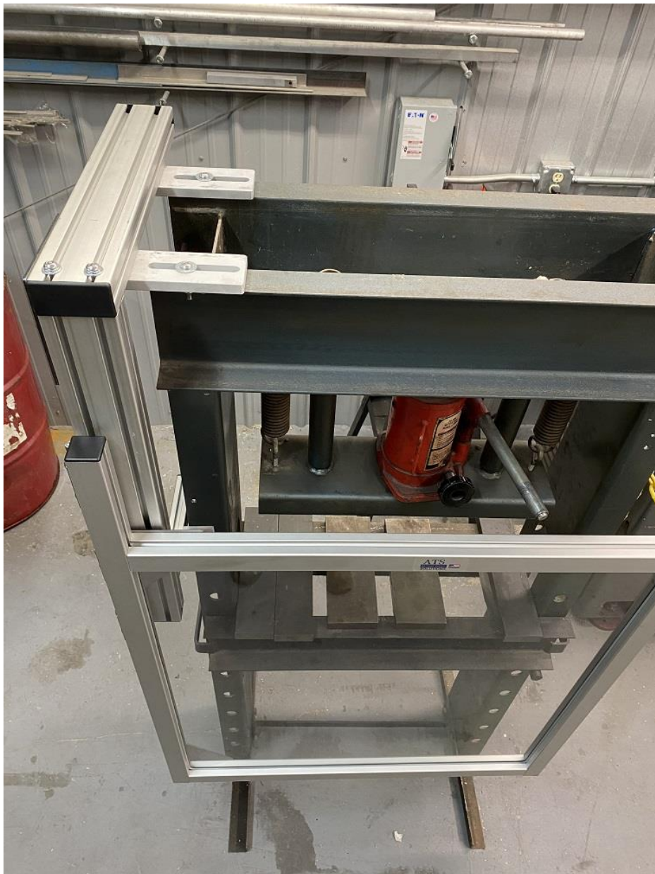
Mounts to the top of the machine with slotted \frac{1}{2} " thick aluminum brackets
