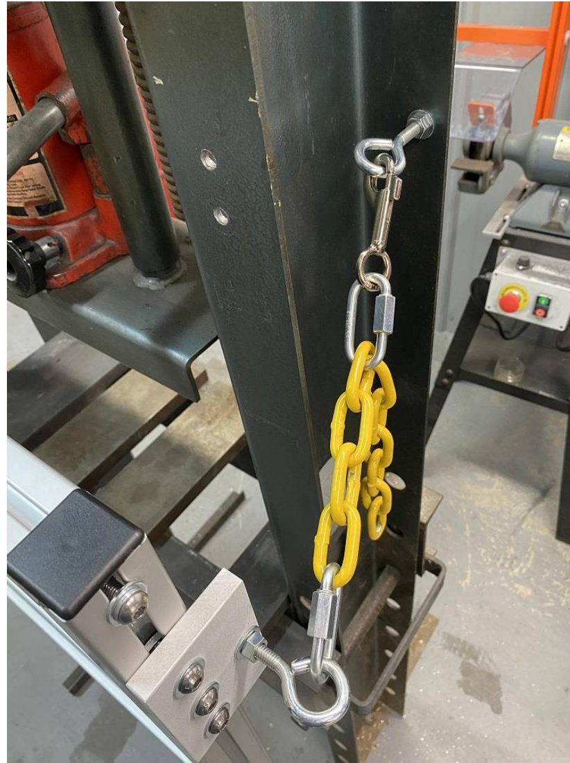
Simple chain and eye bolt setup for keeping the door closed for operation.
