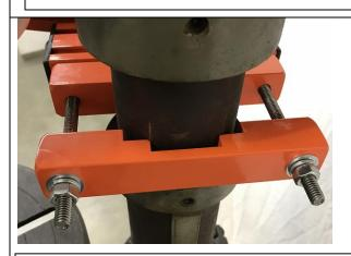
Tighten evenly, using a 1/2" wrench. Snug clamp, but still allow it to rotate.
