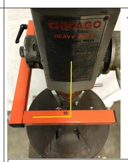
Square the front arm to the machine. Now you may tighten the clamp. Do not over-torque.
