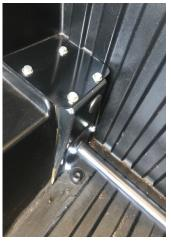
Above is a picture of the shock tower installed with the top cover plate in the correct position
