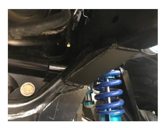
Once you have welded the fill plates in you need to install the cross member gussets. Take your time cleaning the paint off the frame and fit the gussets in. You may need to do some sanding on the stock frame where the factory welds are in order to get the plates to sit flush. When you have the plates fitting up nice you can then burn them in.
