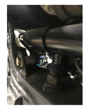
The slide rack end caps have to tabs on them. The top tabs use the factory rack bolts and the front tabs require welding the supplied mounts. Make sure you have the aluminum spacer between the end cap and the tab that gets welded on. Also DO NOT force the tabs into position, this will cause the slide rack to bind. You need to make sure the slide rack is running in parallel to the OE rack.
