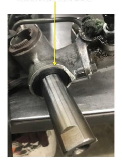
You will need to modify your OEM rack to accept the provided seals. The passenger side uses the machined aluminum seal adapter that slip fits over the OE rack and is locked into place with a set screw. The driver side casting will need to be cut back to accept the provided seal. If you do not cut the rack back then the new clevis will contact the rack before the truck can reach full lock. You will need to cut 1" off the stock rack in order to get the seal to sit flush.
