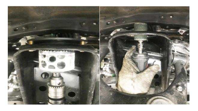
Step 8- If you purchased a secondary shock mount for your LT kit this is the time to install it. After you have opened up the upper shock mounts, bolt the bypass mounts on. To get the bypass mounts to sit flush against the frame you will have to sand down some exposed bolts that protrude through the inner fenders. Once the bypass mounts are bolted up mark where they
