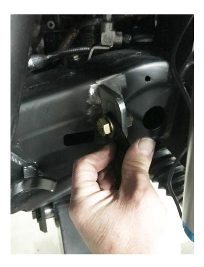
Step 20- The shock reservoir mounts need to be welded to the front portion of the frame rails. We recommend tack welding them on first and checking the fit. Make sure the shock hose does not contact the upper arm when the suspension is completely dropped out.
