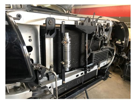
If you are running the reservoir with the filter then you will need to mount it in the location shown below. We supply you with a sandwich plate that allows the bracket to be bolted to the front core support.
