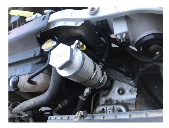
If you are running the reservoir without a filter then it can be installed against the inner fender as seen in the picture to the right.
