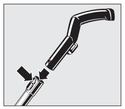
The handle can also be fitted directly to the vacuum cleaner housing.
