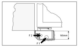
**Note:** while positioning the box, keep in mind the minimum distance there must be between the pillar and the centre of rotation of the gate hinge.
