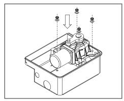
2 • Insert the ball on the box stud and apply the gate anchor (L1).
