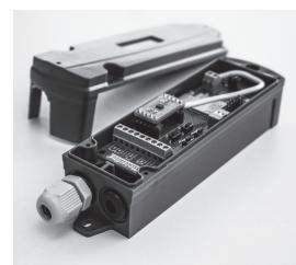
The MX14 is a emitter that communicates wirelessly with the MR14 receiver, up to 50m in the open, powered by batteries or rechargeable batteries by solar panel.
