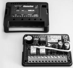
The MR14 receiver is a wireless receiver for managing multiple MX14 emitters. When receiving information from the emitter, it communicates with the automation control board via cable, so that the automation can be stopped or reversed.
