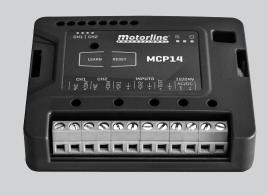
The MPC14 is a controller for 8k2 resistive safety bands and optical safety bands. With its 2 channels, it ensures continuous supervision of the security system and locks it if necessary.
