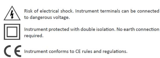
This instrument has been designed and verified conforming to the 61010-1 CE Security Regulation, for industrial applications. Installation of this instrument must be performed by qualified personnel only. This manual contains the appropriate information for the installation. Using the instrument in ways not specified by the manufacturer may lead to a reduction of the specified protection level. Disconnect the instrument from power before starting any maintenance and / or installation action.
