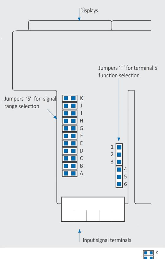
Jumpers not used can be stored for Jumpers stored at future use by placing them at the 'no 'no contact' position contact' positions indicated below.
