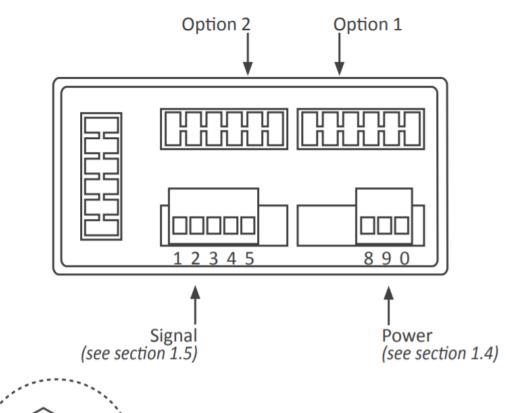
Detail of the plug-in screw terminals provided with the instrument. The instrument is provided with all terminals needed, both male and female.
