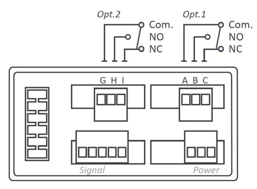
Terminal A, GCommonTerminal B, HNO - Normally openTerminal C, INC - Normally closed
