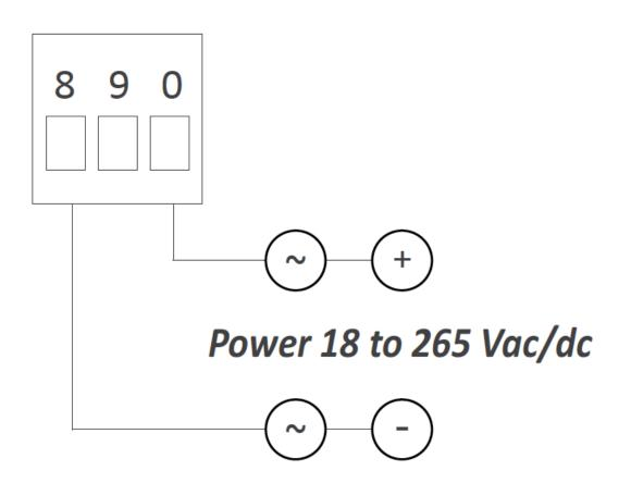
Earth connection - The instrument does not need earth connection for correct operation nor for compliance with security regulations. Terminal 9 is not connected to any internal circuit and is provided only as a safe place for earth wire.
