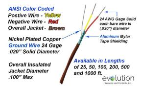
**Type K** Twisted Shielded 24 Gage Solid thermocouple grade wire has a FEP insulation over the bare wire with a temperature rating up to 400°F (200°) although it can accurately transfer the full temperature range of Type K thermocouples.
