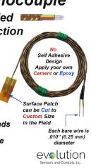
Type K Cement-On Thermocouple Non-Adhesive Surface Patch 30 Gage Bead Welded Thermocouple Junction **Dimensions and Mounting** Instructions 1.00" .1.00" (25 mm) (25 mm) 40 Inches (1 Meter) .750" (19 mm) Surface Tempeature Mounting Polyimide Side Thermocouple Junction Apply Epoxy or Ceramic Cement to this Side Between Layers Apply Epoxy or Ceramic Cement to this Side and Place this Side on the Surface to Measure Fiberglass Insulated Top Side
