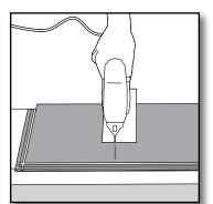
[8] Place the plank face down on the work surface and cut to size with a power saw. If you are using a hand saw, use a fine-toothed blade, and cut the planks face up.
