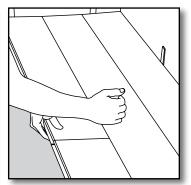
**[6]** If you wish to remove the flooring, just lift the planks a few inches and tap along the joint.
