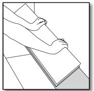
**[5]** Replace the first row by inserting planks from left to right. Press the first board with the groove toward the edge of the planks that are already in position.
