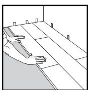
**[12]** The distance to the walls can be adjusted when three rows are completed. Remember to place the flooring a minimum of 1/4" from all walls or other vertical obstructions such as cabinets, pipes, or columns.
