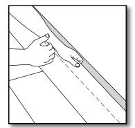
[4] Now remove the first row. Lift the planks a few inches and tap along the joint. Cut the planks as required.
