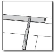
**[15]** Measure and cut the planks in the last row to fit. Remember to allow for a minimum of 1/4" expansion space from the wall.
