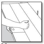
**[13]** You may have to disassemble the flooring due to obstructions, etc. Just lift the row of planks a few inches and tap along the joint.
