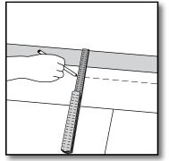
**[11]** If the starting wall is uneven, the planks must be adapted to its contours. You can scribe the contour of the wall onto the first row of planks by using a ruler and a pencil to follow along the contour of the wall. Do not forget to allow for the minimum 1/4" expansion space from the wall. Disassemble the first row, cut the planks along the line you have drawn, and then reassemble. You must still use the spacers to maintain the expansion space along this wall.
