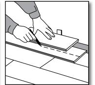
**[16]** Use a full width scrap plank to mark your cutting line on the last row.
