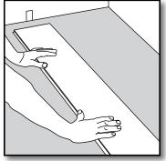
**[1]** Assemble three or four rows well away from the starting wall. Begin by placing the tongue of the short plank toward the starting wall.
