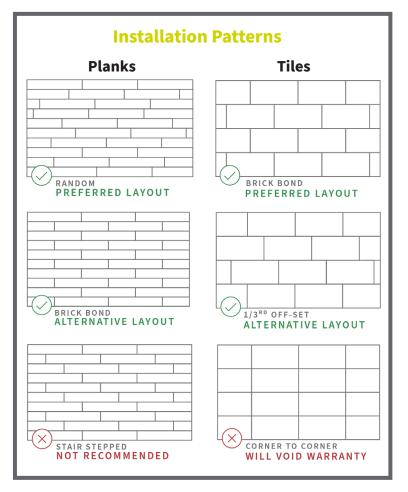
**Layout:** Prior to installation, confirm the installation pattern and direction per the design specifications or work order. Planks should be installed in a random pattern - plank end joints should be randomly spaced by ≥ 8-in. Avoid "H" joints and do not install in a "Stair Stepped" installation pattern, while ensuring no obvious pattern repeats emerge. Tiles should be installed in a brick-bond or
