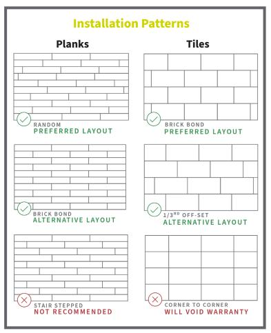
to failure. Tiles must be installed in a brick-bond or 1/3rd off-set
