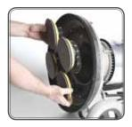
2) Tip the machine backwards and remove the dust skirt.
