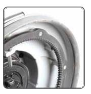
**4)** To remove the Power Drive<sup>™</sup> drive plate, turn the paddle lever so it is in the unlocked position (A). Place the tip of the supplied box spanner between the driving axle and drive plate bracket, then push against the drive plate to release the interlock (B). Turn one of the sanding discs counterclockwise until the drive plate can be freed.
