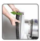
Always remove the dust skirt and the drive plate or sanding disc before transportation. Always vacuum and clean machine after use. When transporting the machine via vehicle, make sure that the machine is securely fastened through the wheels to avoid movement.
