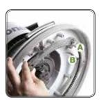
**3)** To install the Power Drive<sup>™</sup> drive plate, place the drive plate into position and turn it to engage the interlock (*A*). Once it is in place, turn the small flat paddle lever (*B*) to make sure that it is bolted into place.
