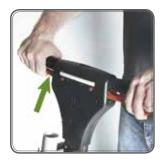
If the machine becomes difficult to handle, release the start handles and the machine will stop immediately.
