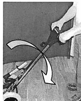
2. Lower the handle shaft to the desired position. The lower position with relaxed arms, the easier the machine will be to handle. Release the button.
