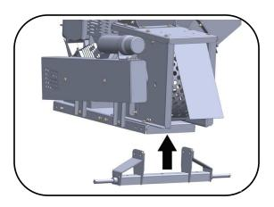
First, assemble the two trailer brackets as shown. Then, assemble the tow bar below the brackets, as shown on the same figure. For this operation, 2-3 person assembly team is recommended.
