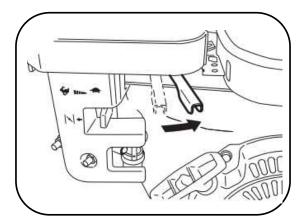
**2.** Turn the engine switch OFF and close the fuel access; figures shown below.
