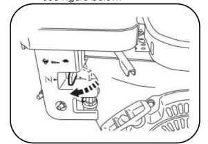
**3.**Move the lever throttle control to the center position between idle and fast. See the figure below.
