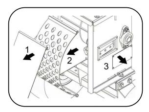
**NOTE:** To remove the blade's bolts, it is recommended to place a piece of wood in between the rotor and the outside edge to prevent it from rotating when applying torque on the nuts from the back.
