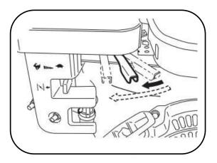
**4.** Firmly hold the handle of the starter rope, pull the starter cord slowly until resistance is felt, then pull rapidly.
