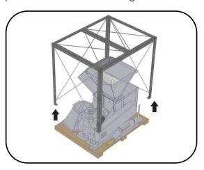
**4.** Remove the chipper by removing the platform anchor plates. See Fig. below.
