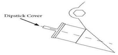
**NOTE**: The engine is shipped without oil. Operating the engine with no oil or oil at a low level will destroy the engine. This is **not** covered under warranty.
