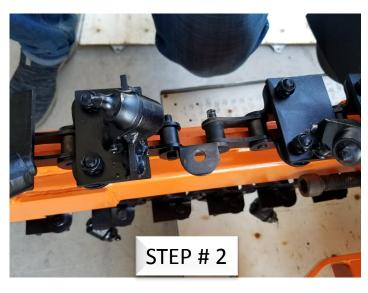
INSTALL CHAIN PLATE WITH PINS
