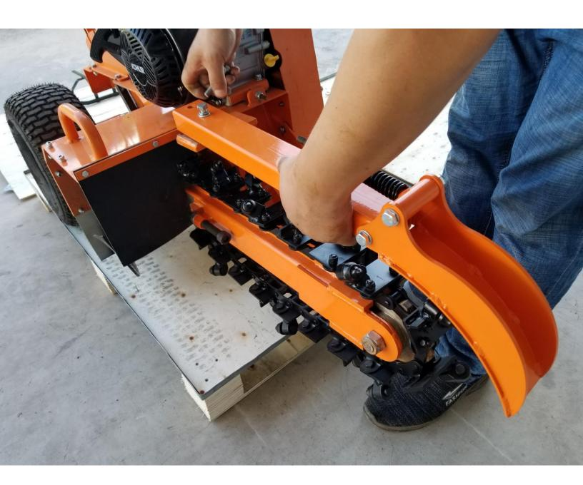
1. INSTALL AUGER GUARD WITH BOLTS PROVIDED IN THE MOUNTING HOLES.
