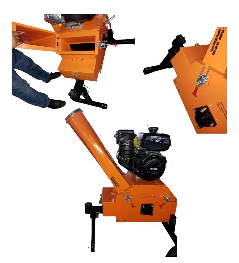
1. Install the Chip Chute Directional Deflector and tighten the locking handles.
