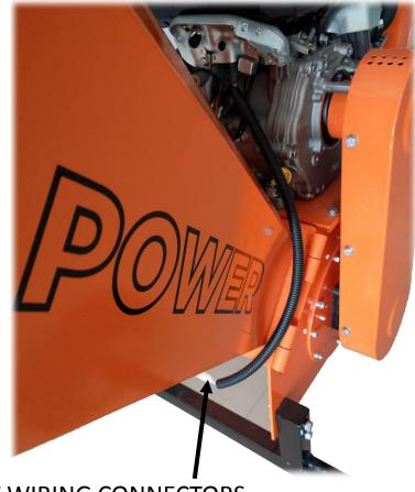
CONNECT WIRING CONNECTORS
