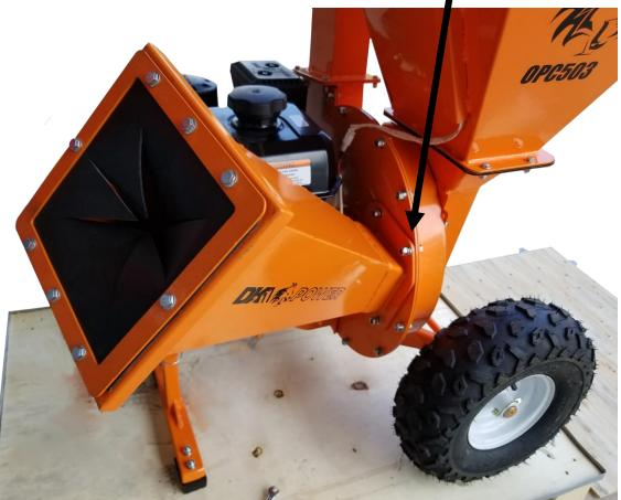
1. INSTALL THE HANDLE USING 4 BOLTS PREINSTALLED ON THE CHUTE FOR THE HANDLE TO BE ASSEMBLED.
