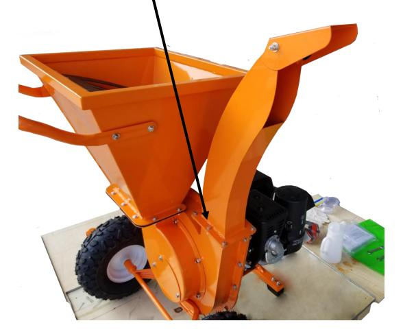
1. Mount the FEED CHUTE onto the Chipper using supplied bolts and hardware.
