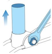
3 Loosely tighten the lateral nuts on either side of the bike seat.
