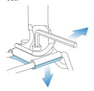
Take your new bike seat and mount the seatpost onto the rails. Then loosely screw the bolt(s) using the hex key.
