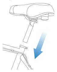
5 Ensure the bike seat is parallel to the ground. Then tighten the bolt(s) using the hex key. Once it's securely fixed to the seatpost, go for a test ride.
