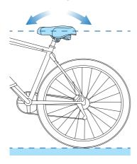
6 When the desired angle is found, use the wrench to securely tighten the lateral nuts on either side of the bike.
