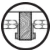
The Above shows a cross section of a side wall with 2"x 6" pine 16" OC , 1/2" ply , R11 batt with a 3/4 " airspace between the Batt and ArcticShield™ as well as 3/4" space between interior wall and ArcticShield™ using staple tabs to secure.
