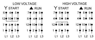
FULL VOLTAGE ACROSS THE LINE START AND RUN ON A CONNECTIONS. ALSO SUITABLE FOR START ON Y, RUN ON A.
