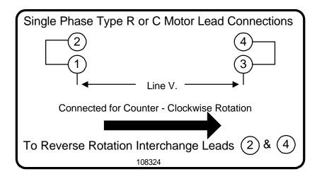
Motors are connected for counter clockwise rotation. To reverse direction of rotation, interchange leads 2 and 4.
