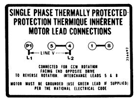
Connected for CCW Rotation Facing End Opposite Drive. To reverse direction of rotation, interchange leads 5 & 8.
