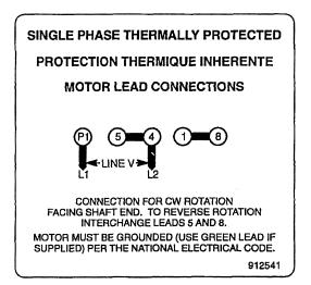
Connected for CW Rotation Facing the Shaft End.
