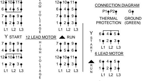
FULL VOLTAGE ACROSS THE LINE START AND RUN ON  $\triangle$  CONNECTION. ALSO SUITABLE FOR START ON Y, RUN ON  $\triangle$  .
