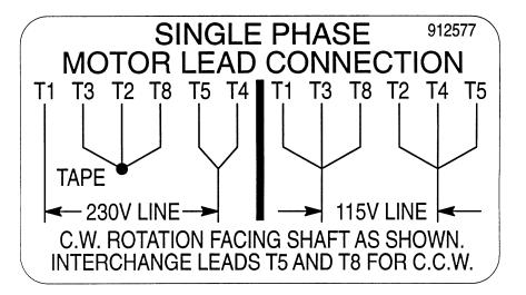
Connected for CW Rotation Facing Shaft End.
